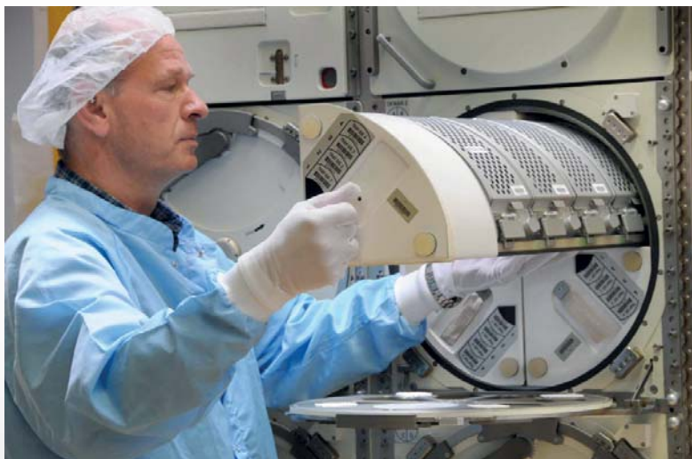
The third unit of the minus 80 degree freezer (MELFI) under testing. Image: Astrium GmbH/Alfred Rutloff.
